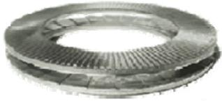
NORD-LOCK is a pair of washers with a wedge-locking action meeting DIN 25201 which is a unique method using tension instead of friction. The rise of the cams between the NORD-LOCK washers is greater than the pitch of the bolt. In addition, there are radial teeth on the opposite side. The washers are installed in pairs, cam face to cam face.
